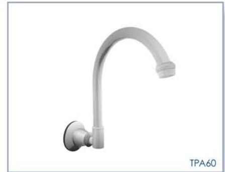
PASADENA WALL SPOUT Overall Height = 210mm Spout Height = 135mm BASE TO AERATOR Spout Length = 140mm 4 Star Water Efficiency Rating
