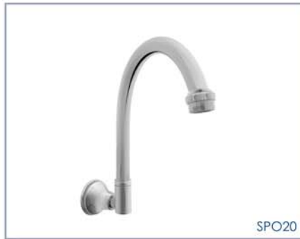
DALLAS WALL SPOUT Overall Height = 215mm Spout Height = 140mm BASE TO AERATOR Spout Length = 230mm 4 Star Water Efficiency Rating
