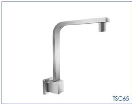
CUBA WALL SPOUT Overall Height = 205mm Spout Height = 165mm BASE TO AERATOR Spout Length = 180mm 4 Star Water Efficiency Rating
