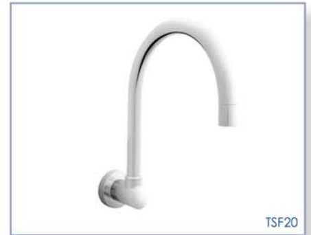
WALL SPOUT Overall Height = 220mm Spout Height = 115mm BASE TO AERATOR Spout Length = 205mm 5 Star Water Efficiency Rating
