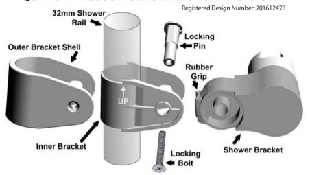
**QUIK-GRIP Handy Hint:** Locate the UP symbol on the Inner Bracket to guarantee alignment of all components during installation.
