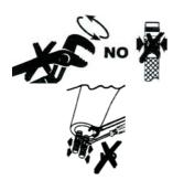
Never use tools to install or remove hoses as this may damage the hose and the plumbing fittings.
