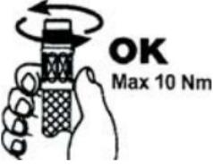
Install hose using hand pressure not exceeding 10Nm. Always hold the fitting end when installing the hose never twist the hose.
