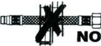
Never install a braided hose through or behind walls, in inaccessible locations or places where the hose can not be visually inspected.
