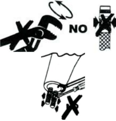
Never use tools to install or remove hoses as this may damage the hose and the plumbing fittings.
